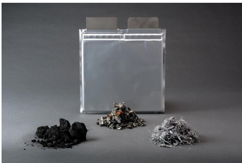
Image 2 shows a pouch cell and materials recovered during the recycling process. Courtesy of Argonne Laboratories.
